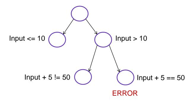
Path constraint is a conjunction of constraints along a path from root of the tree to a leaf node
